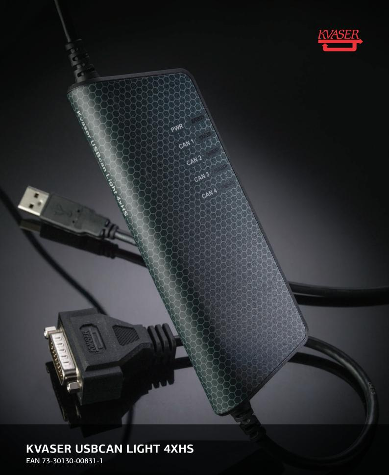
The USBcan Light 4xHS is a compact, reliable and cost-effective means of connecting four high-speed CAN busses to a PC or mobile computer. With galvanic isolation as standard, this USB to quad channel CAN interface has a standard USB connector at one end and four high speed CAN channels in a single 26-pin HD D-SUB CAN connector at the other. The supplied HD26-4xDS9 splitter can be used to connect to four separate 9-pin D-SUB connectors.
