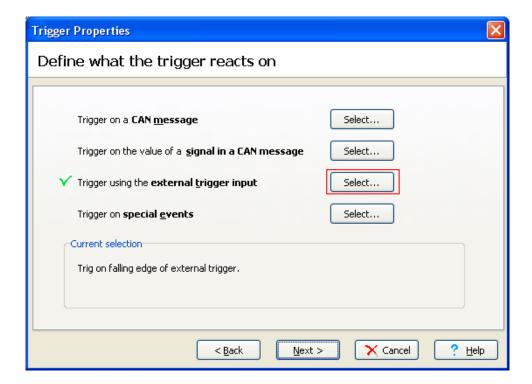
Figure 11. Selecting external trigger.
