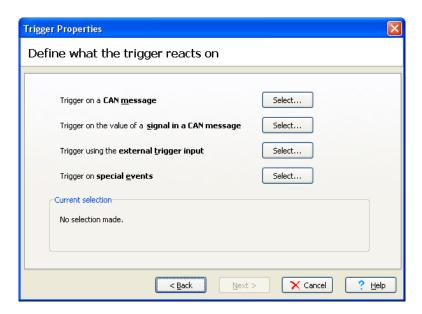
Figure 3. Selecting trigger types.
