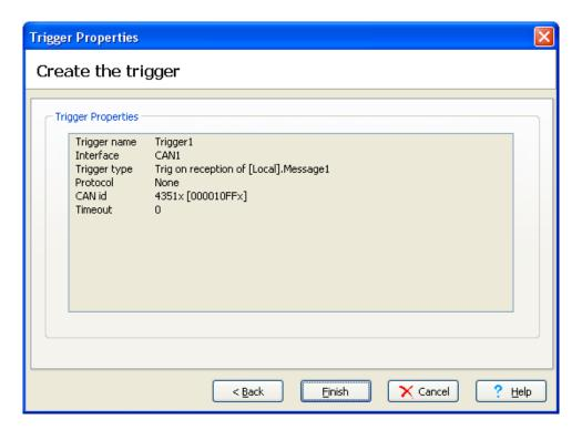
Figure 5. Trigger properties.
