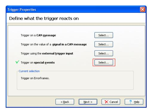
Figure 9. Selecting Error Frame trigger.
