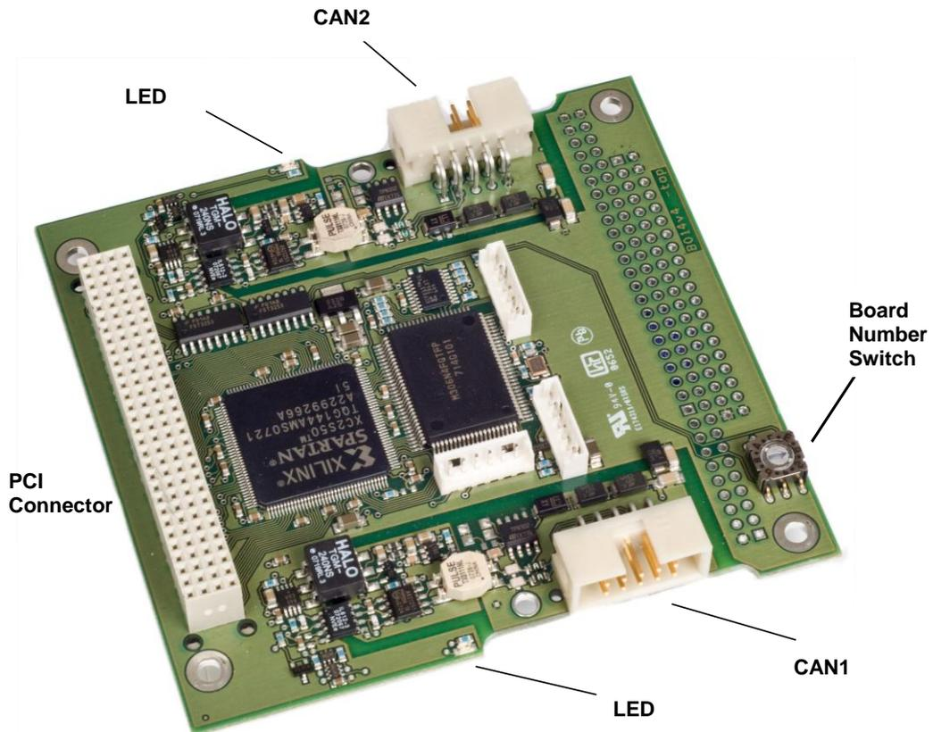
Figure 1: Connectors and switches on the Kvaser PCI104.
