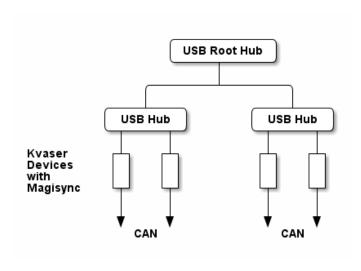
Figure 6: An example setup where all devices are synchronized via MagiSync.
