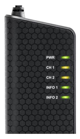
Figure 4: LEDs on the Kvaser Hybrid Pro 2xCAN/LIN.
