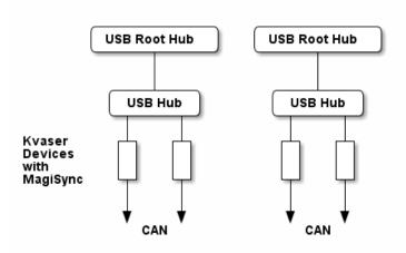
Figure 7: Not all devices are synchronized via MagiSync in this setup.
