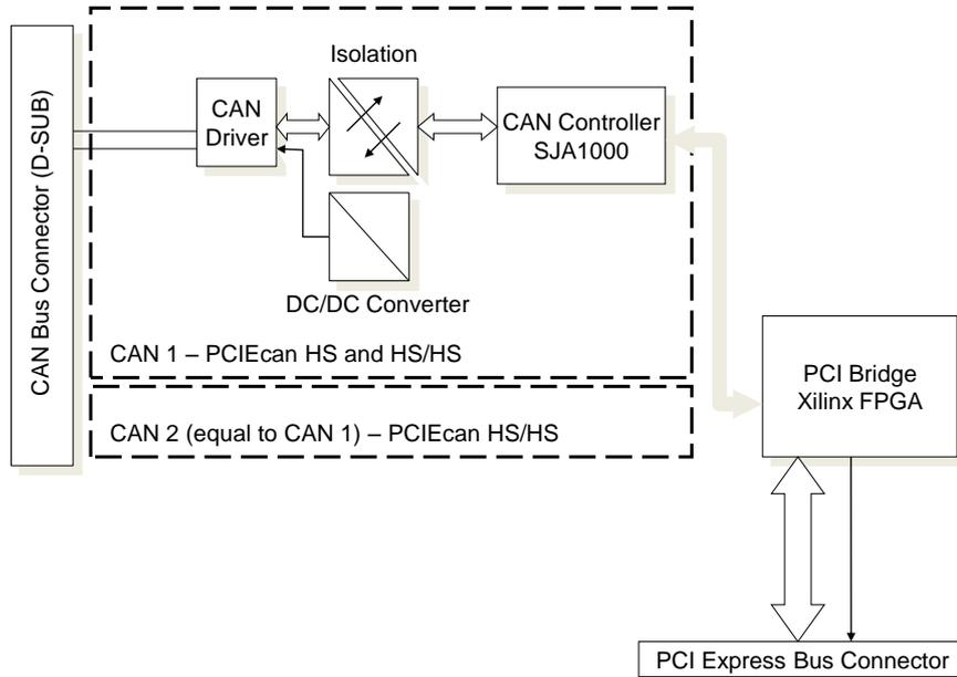
Figure 1 Block diagram for Kvaser PCIEcan HS/HS.
